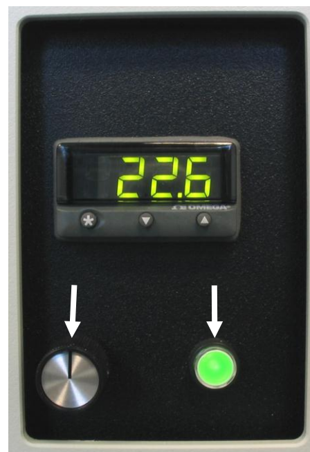
The SPRImager®II control panel (above) showing the pump rate control (left arrow) and pump On/Off switch (right arrow).
