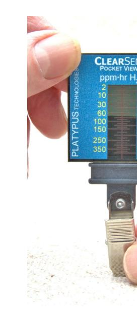
The dosimeter clips onto clothing (left) for personal monitoring and can be read in ambient light with the zero-power Pocket Viewer (middle), or with the ClearSense<sup>™</sup> USB reader (right) connected to a computer.
