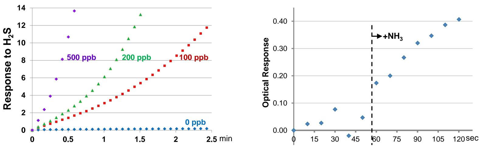
*Fast Response Sensors*: Left, H<sub>2</sub>S sensor responses to 0-500 ppb target. Concentrations down to 100 ppb are detected within a minute, and response rates are a function of target concentration, i.e. the sensors are quantitative. Right, NH<sub>3</sub> sensor response to 100 ppb target again is measurable within a minute.
