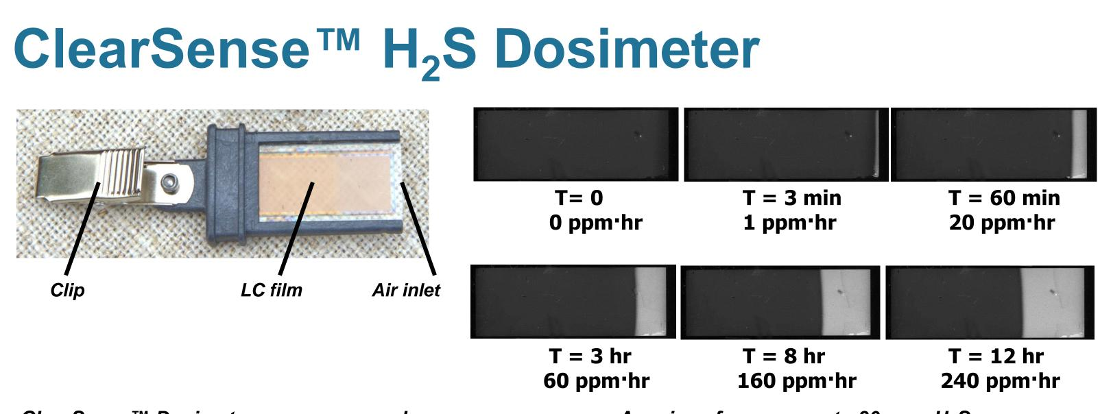
ClearSense™ Dosimeter, cover removed
