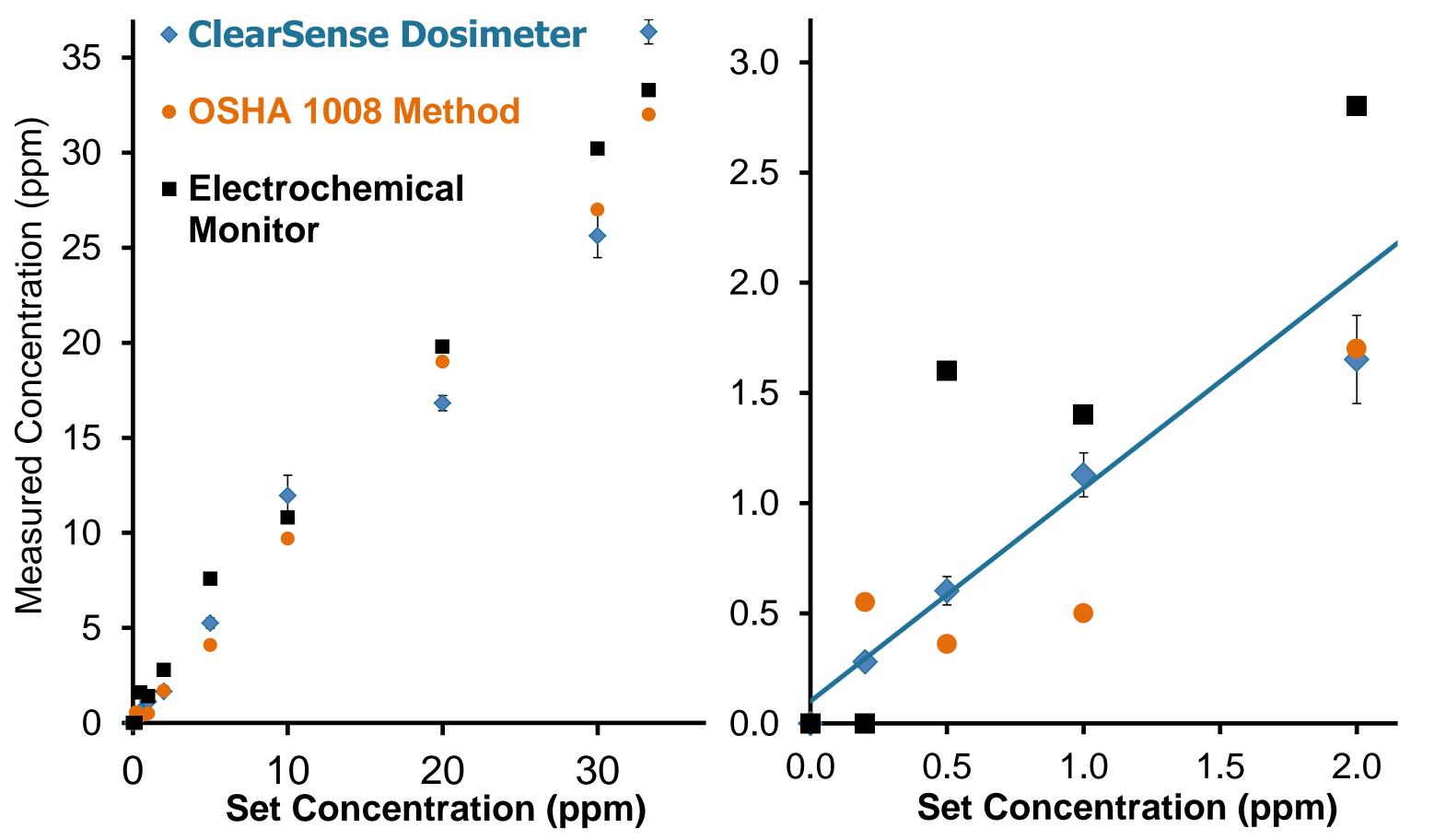
Laboratory validation of ClearSense<sup>™</sup> Dosimeters. Five dosimeters each were exposed to nine different concentrations (0.2 to 33.3 ppm) of  $H_2S$  for different durations (15 min. to 12 hr.) at 60% RH. Using an algorithm, the concentrations were determined and compared with the concentrations measured using an EC Monitor and the OSHA-1008 method.
